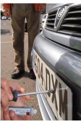
and replacing them with clutch-head screws. These are screws that can only be turned clockwise and you need a drill to remove them. Stick-on plates are never a good idea – they can be removed quickly and quietly. Visit www.secureplate.com for details on tamper-proof index plates. Many garages offer to fit anti-theft plates: please check the product is dvlaapproved and bears the 'Sold Secure' logo. Many non-tested products are proving not to work effectively.
